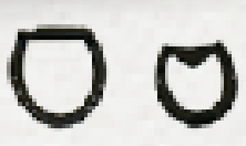
Handmade stirrups, fashioned from horseshoes, made for dudes so their feed would not slip through the stirrups and cause them to be dragged by their horse if they fell off while riding.
